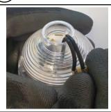
(a). Push connection points to one side to gain access to circuit board.
