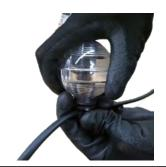
(d). Visually check the seal has not been trapped and is in good condition. In a clockwise twisting direction, lock and click the globe to the festoon cable.
